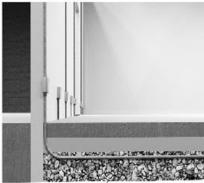
Detail 1 – Heating cable in 3/4" rigid conduit
